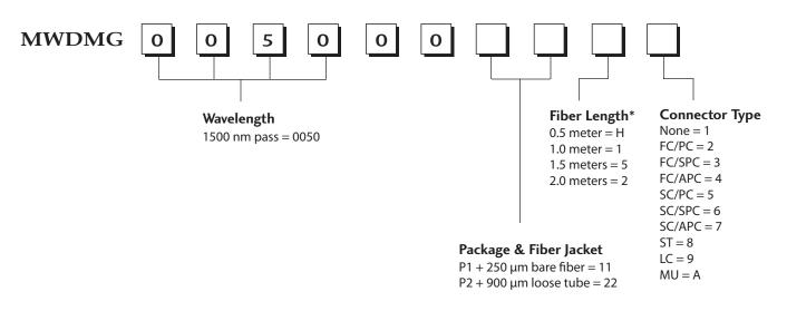
\* The tolerance of fiber length is +/-0.1m. 1 meter is standard. The lead-time for special fiber length will be longer.
